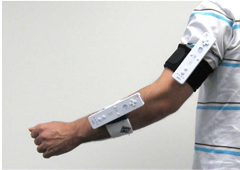
Figure 2.10. Using a second Wii remote attached to the upper arm to detect and cancel out compensatory motions.
