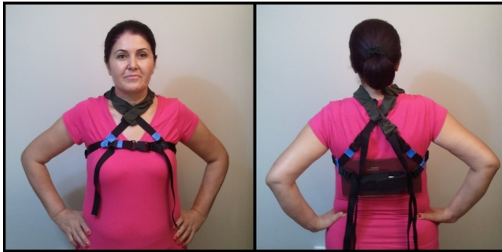
Figure 6.4. The harness we designed to track the torso motion with a Wii remote. The pocket that holds the Wii remote is attached to the rectangular brown cardboard piece.
